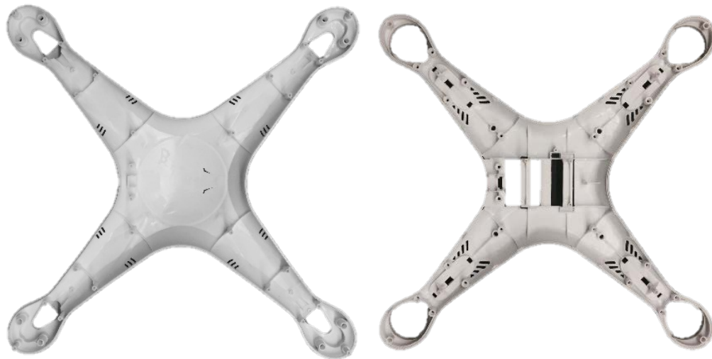
Figure 6-1 - Upper shell (left) and lower shell (right) of the Syma quadcopter in the orientation it was used on the planar optical CMM
