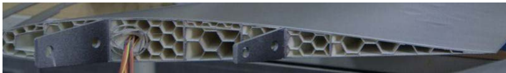
Figure 2-1 Internal structures within an additive manufactured part
